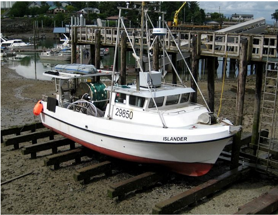
(← Wrangell tidal grid. This owner drove his boat on the grid, waited for the tide to fall, roll-painted his hull and bottom, and then floated off at high tide. He says “Who needs a Travel Lift!”)
